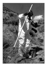
Protective clothing was needed to check groundwater contamination levels at this landfill.
