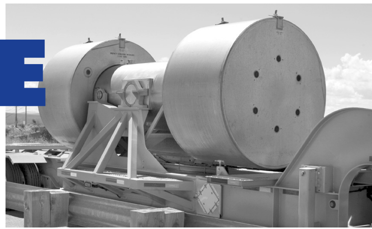
Specialized container used to transport Remote-Handled (RH) waste to WIPP.
