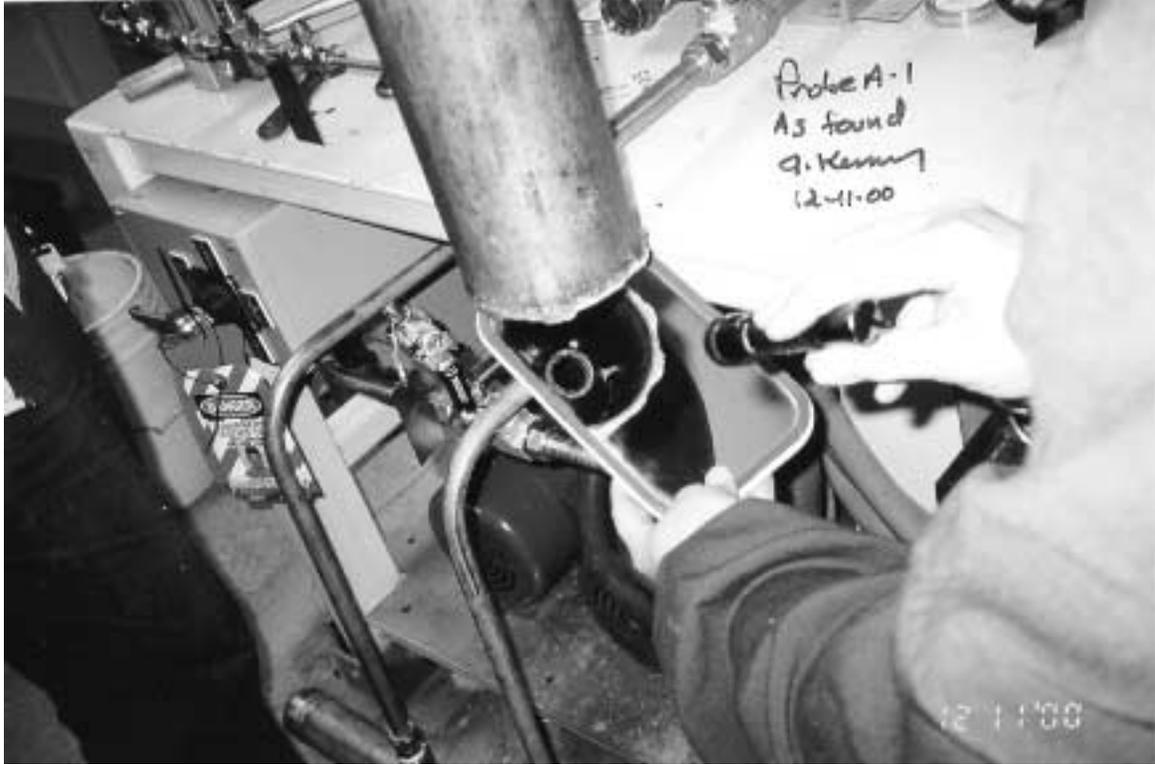
Figure 3. Probe A-1 as found on December 11, 2000. The inner annulus, while not completely clean, is much less occluded than that seen on Probe A-3.
