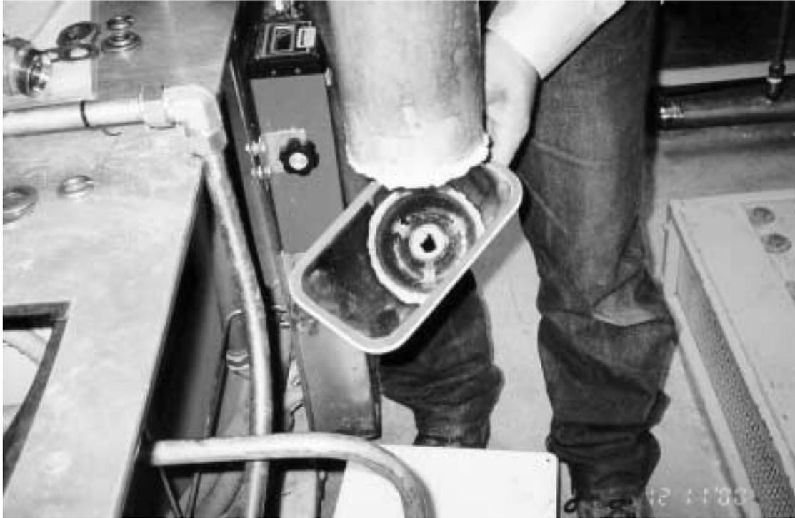
*Figure 2. Probe A-3 as found on December 11, 2000. Samples are taken through the innermost opening shown here, representative sampling requires less than 2 mm on this orifice (Farthing 1989).*
