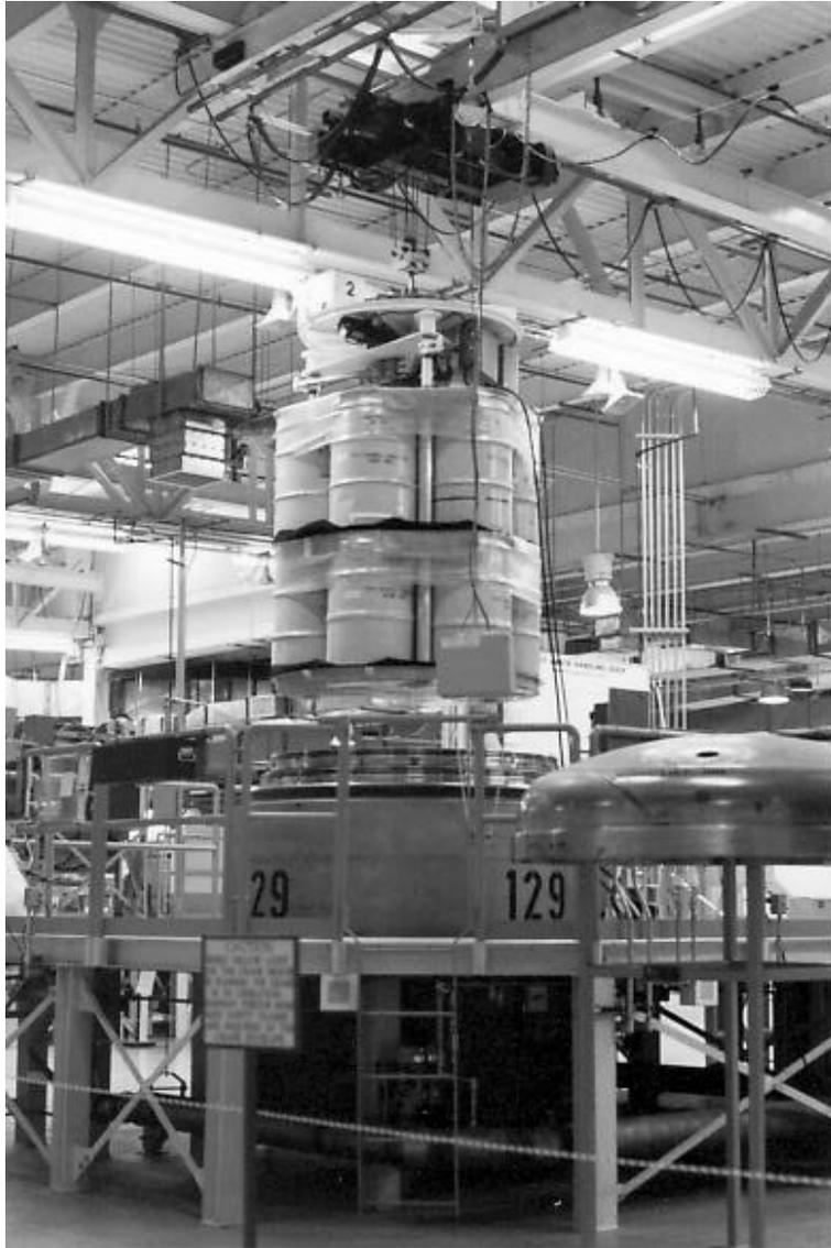
*Picture 3. A waste-handling-bay crane is lifting a 14-drum pack with simulated waste from the TRUPACT-II.*
