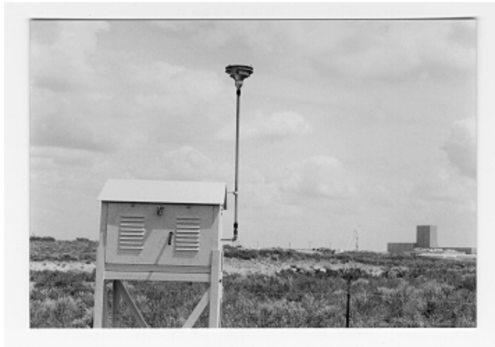
Figure 6. Typical WIPP Site Low Volume Air Sampling Station (S-3)
