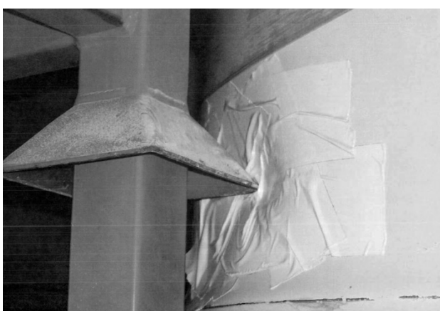
A 55-gallon drum was damaged during emplacement. It was patched in place.
