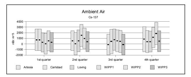
Figure A9. <sup>137</sup>Cs Measurements in LVAS Samples During 2002
