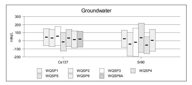
Figure B2. <sup>137</sup>Cs and <sup>90</sup>Sr Measurements in Groundwater During 2002
