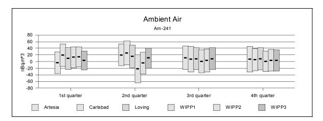
Figure A5. <sup>241</sup>Am Measurements in LVAS Samples During 2002
