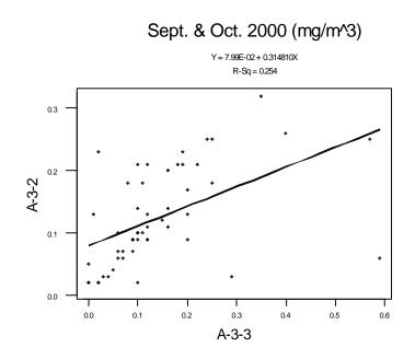
Figure 7. Comparison of mass collected on legs A-3-2 (CEMRC sample) and A-3-3 (EEG sample) during September and October 2000. An "R-Sq" (coefficient of determination) of 1 would represent a perfect correlation between legs.
