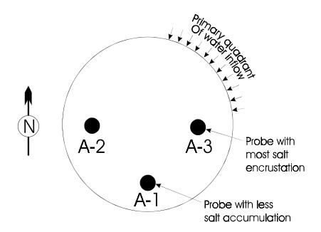
Figure 4. Location of Station A sampling skids at top of exhaust shaft.
