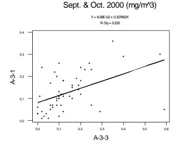
Figure 6. Comparison of mass collected on legs A-3-1 (MOC sample) and A-3-3 (EEG sample) during September and October 2000. An "R-Sq" (coefficient of determination) of 1 would represent a perfect correlation between legs.
