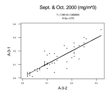
Figure 5. Comparison of mass collected on legs A-3-1 (MOC sample) and A-3-2 (CEMRC sample) during September and October 2000. An "R-Sq" (coefficient of determination) of 1 would represent a perfect correlation between legs.
