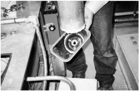
Figure 2. Probe A-3 as found on December 11, 2000. Samples are taken through the innermost opening shown here, representative sampling requires less than 2 mm on this orifice (Farthing 1989).
