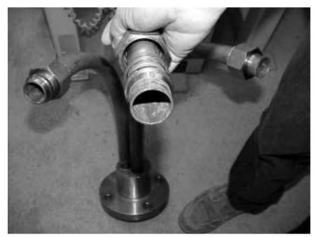
*Figure 12. Skid A-3 three-way splitter and transport line to filter housing (1999)*
