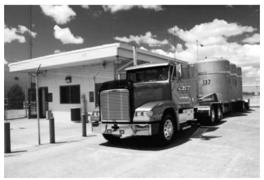
*Picture 4. Three TRUPACT-II shipping containers with simulated waste arrive at the WIPP security gate for inspection.*
