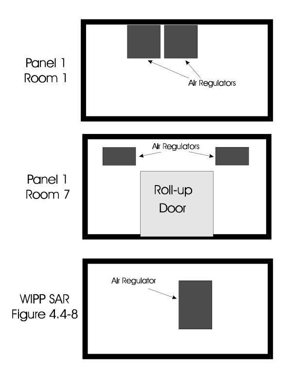
Figure 2. Relative Positions of Air Regulator Louvers in Waste Room Bulkheads
