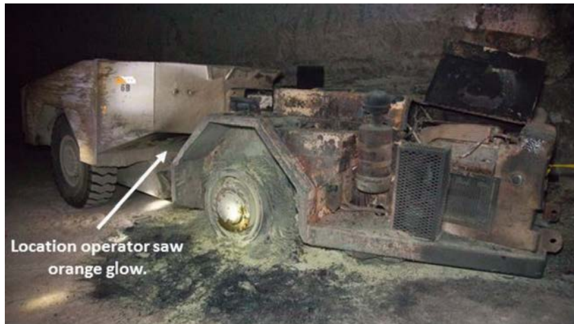
Salt Truck after the fire (Source: DOE)
