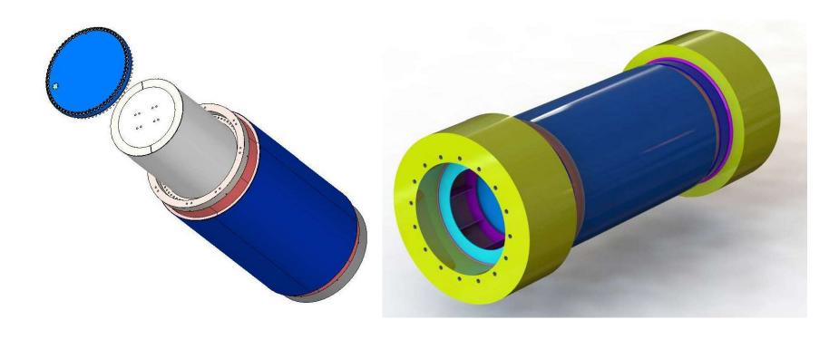
Cask length = 15' 9"/17' 8" Internal Diameter = 6'4" Outer Diameter = 8'10"
