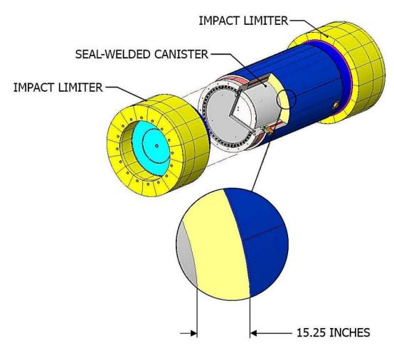
Cask length = 15' 9"/17' 8" Internal Diameter = 6'4" Outer Diameter = 8'10"
