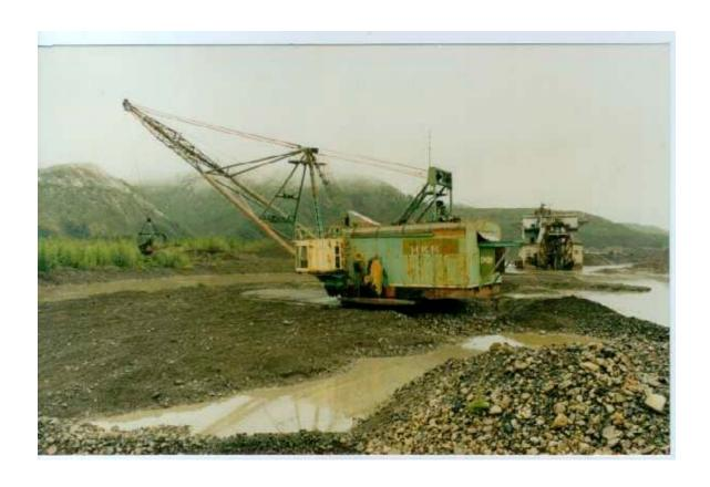
Inactive Mining Equipment – Dragline (left) and Dredge (right) – From Magadan Center for the Environment (MACE), 2002
